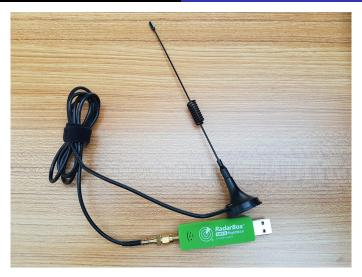
Figure: A USB-receiver which is capable of processing ADS-B (*Automatic Dependent Surveillance-Broadcast*) radio transmissions.
